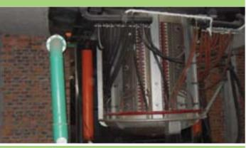
New PP Spunbond non-woven line with heat induction loop technology
